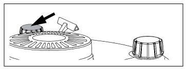
Figure 34. Oil Fill Cap/Dipstick
