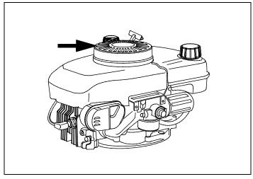
Figure 1. Typical Flywheel Guard Location
