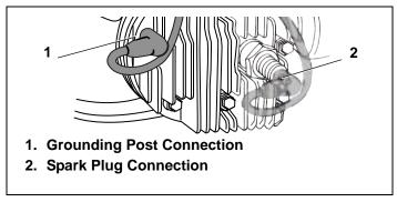
Figure 44. Typical Grounding Post/Spark Plug Connection
