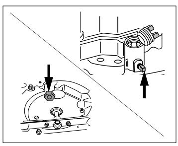
Figure 41. Oil Drain Plug Locations
