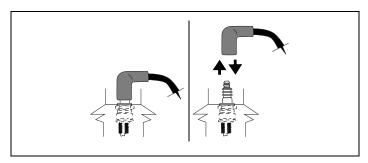
Figure 35. Disconnecting/Connecting Spark Plug
