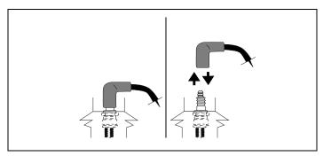
Figure 28. Disconnecting/Connecting Spark Plug
