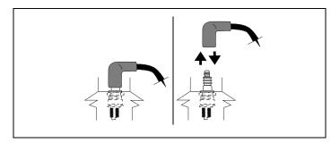
Figure 30. Disconnecting/Connecting Spark Plug
