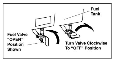
Figure 11. Fuel Valve Positions
