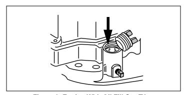
Figure 9. Engine With Oil Fill Cap/Plug
