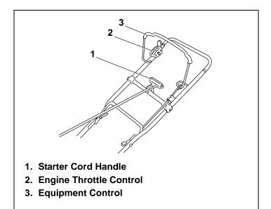
Figure 25. Typical Engine Controls
