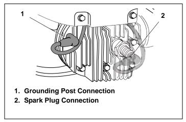
Figure 39. Typical Grounding Post/Spark Plug Connection
