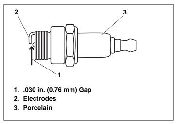
Figure 47. Resistor Spark Plug
