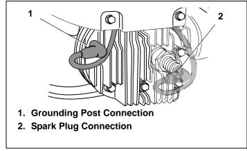
Figure 54. Typical Grounding Post/Spark Plug Connection
