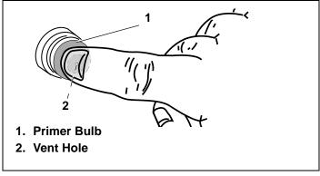
Figure 20. Pressing Primer Bulb
