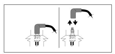
Figure 2. Disconnecting/Connecting Spark Plug
