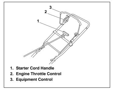
**Figure 21. Typical Engine Controls**
