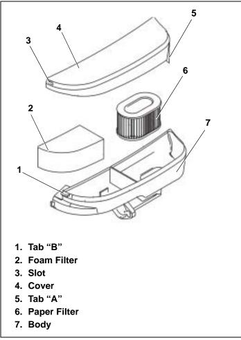
Figure 51. Air Cleaner Type "D" Assembly
