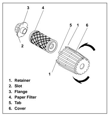
Figure 50. Air Cleaner Type "C" Assembly
