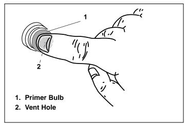
Figure 14. Pressing Primer Bulb
