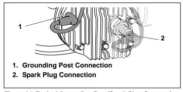
Figure 31. Typical Grounding Post/Spark Plug Connection
