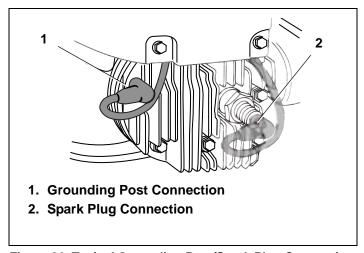
Figure 36. Typical Grounding Post/Spark Plug Connection
