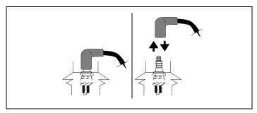
Figure 43. Disconnecting/Connecting Spark Plug
