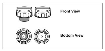
Figure 10. Possible Fuel Fill Cap(s)
