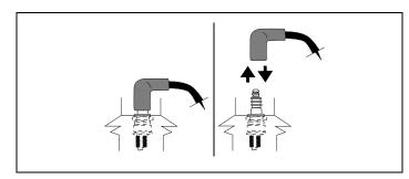
Figure 38. Disconnecting/Connecting Spark Plug
