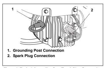
Figure 3. Typical Grounding Post/Spark Plug Connection
