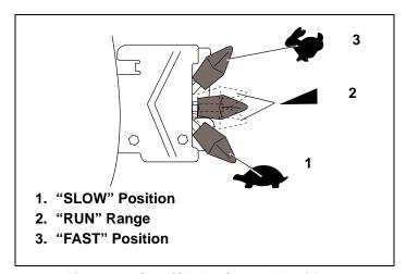
Figure 19. Start/Choke Control Positions
