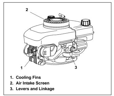
Figure 46. Debris Removal Locations
