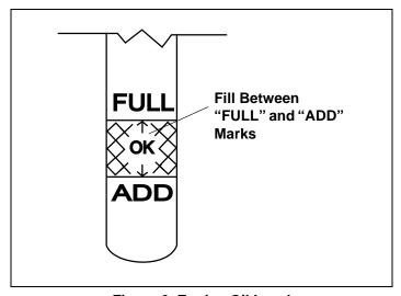
Figure 6. Engine Oil Level
