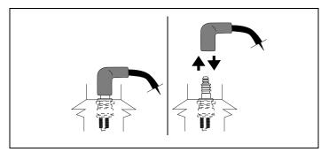
Figure 53. Disconnecting/Connecting Spark Plug
