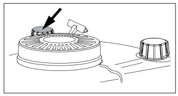
Figure 8. Oil Fill Cap/Dipstick
