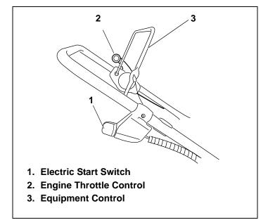
**Figure 12. Typical Engine Controls**
