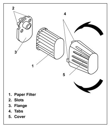
Figure 52. Air Cleaner Type "E" Assembly
