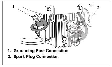
Figure 29. Typical Grounding Post/Spark Plug Connection
