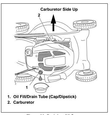
Figure 33. Draining Oil Sump
