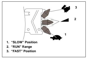
Figure 16. Start/Choke Control Positions
