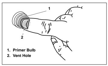
Figure 24. Pressing Primer Bulb
