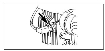
Figure 37. Typical Spark Plug Connection
