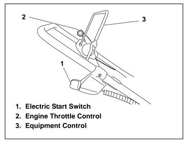
**Figure 17. Typical Engine Controls**
