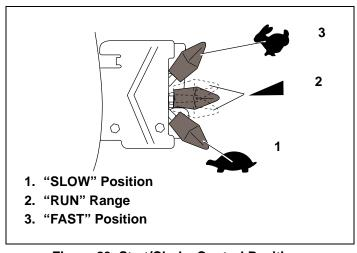
Figure 23. Start/Choke Control Positions
