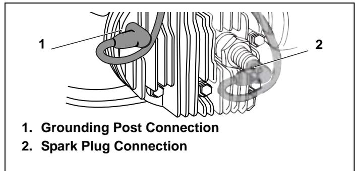
**Figure 44. Typical Grounding Post/Spark Plug Connection**
